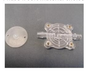
Phase II: membrane sensorization hypothesis (thickness 220nm)
